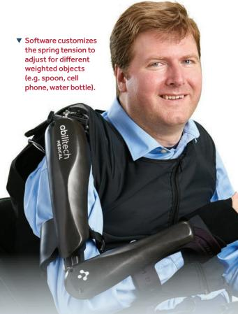
▲ Springs at the shoulder and elbow support the users' existing strength for smooth and natural movement of the arms.
